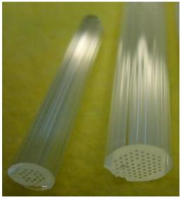
Single-mode large mode area photonic crystal fibers combine a large effective mode filed area and relatively low loss to allow high average/peak power delivery without nonlinear effects or material damage over long distances.
