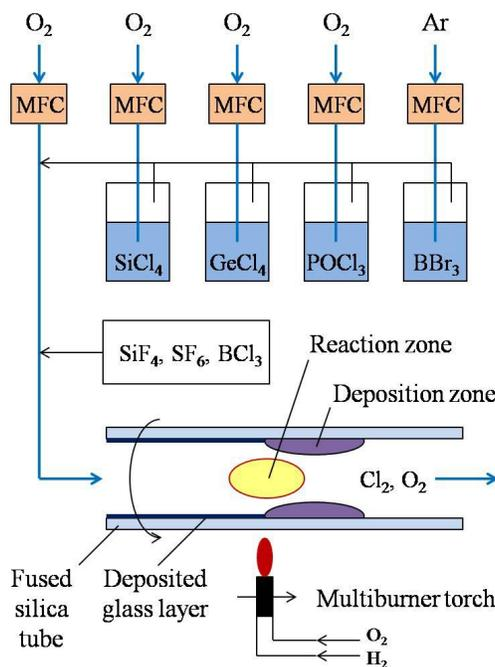
Figure 1. The process of silica optical fiber preform fabrication by the MCVD method.
