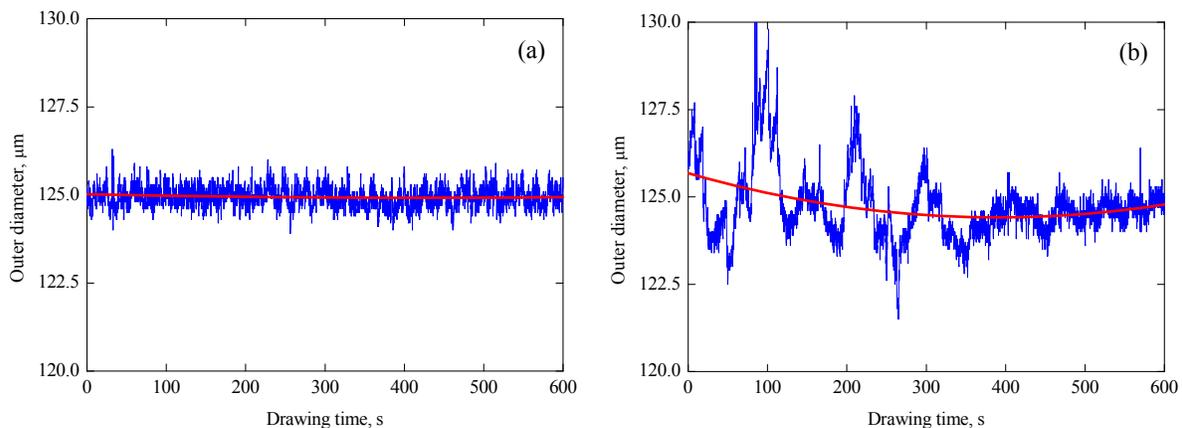
Figure 4. Indications of the outer diameter of MMFs drawn (a) under the automatic stability maintenance and (b) under the manual stability maintenance.
