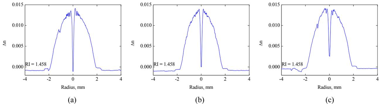
Figure 2. Measured RI profiles of the first series MMF preforms with the depth of the dip (a)  $\Delta n_d = 0.015$ , (b)  $\Delta n_d = 0.014$  and (c)  $\Delta n_d = 0.0115$ .
