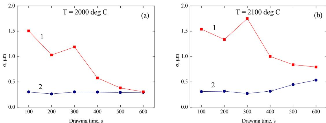
Figure 5. The standard deviation of the outer diameter of MMFs drawn at different temperatures (1) under the manual stability maintenance and (2) under the automatic stability maintenance.
