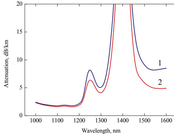
Figure 6. Spectral dependence of attenuation for the samples (1) A-3 and (2) A-1.
