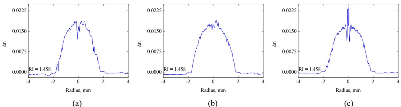
Figure 3. Measured RI profiles of the second series MMF preforms with the depth of the dip (a)  $\Delta n_d = 0.002-0.003$ , (b)  $\Delta n_d \sim 0$  and (c)  $\Delta n_d = -(0.004-0.005)$ .
